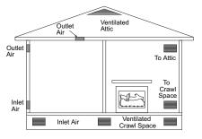
Figure 3 - Ventilation Air from Outdoors
